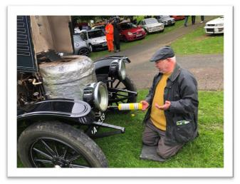
One very interesting vintage car looked magnificent although when I first saw someone pop a lighted blow torch under the front of the car it looked very disturbing. It turned out to be a Stanley steam car and its owner was putting light to a mixture of petrol and diesel twenty minutes before he planned to drive up the hill so was preparing to get up steam.
